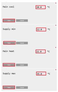
When adjusting on the return temperature we need to set the desired temperature on the Main cool or Main heat item after which we need to set the threshold below which we do not want to go in case of Cool (supply min) on the supply temperature and the threshold above which we do not want to go in case of Heat (supply max) also on the supply temperature.
