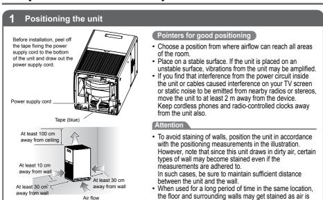
drawn into air inlets near the base of the unit. It is recommended to clean the unit periodically.
