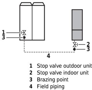
Recovery/vacuuming overview for 1 indoor unit maintenance (R410A circuit connections)
