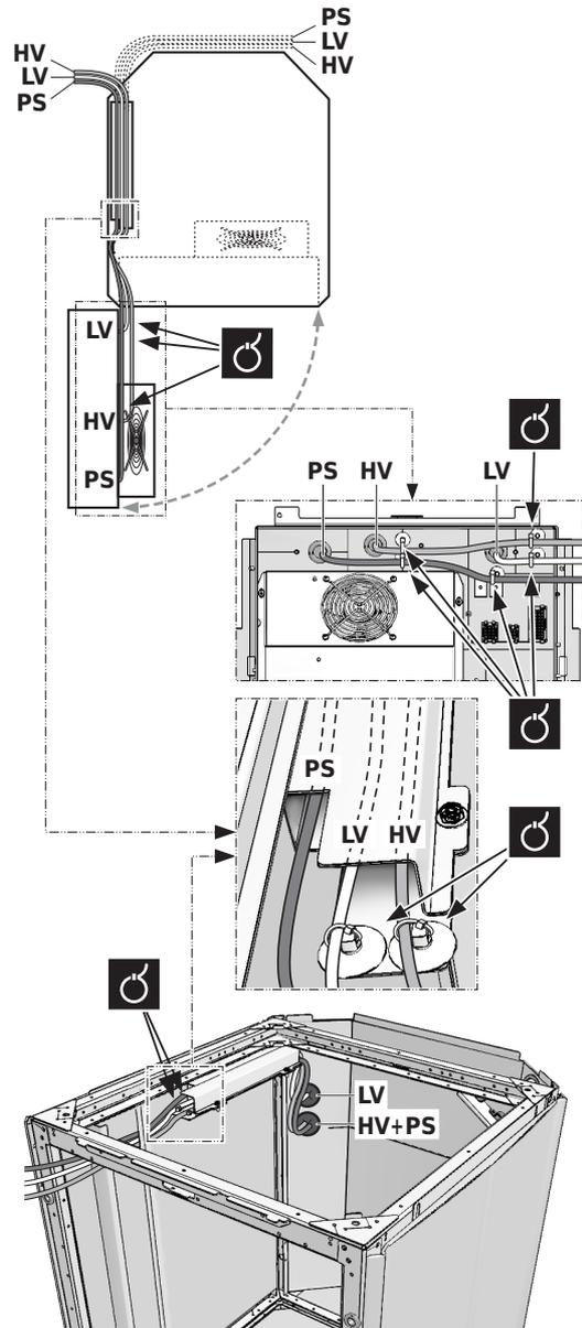
To avoid electric noise problems, be sure that cables are put in the correct bundle as mentioned on the figure.
