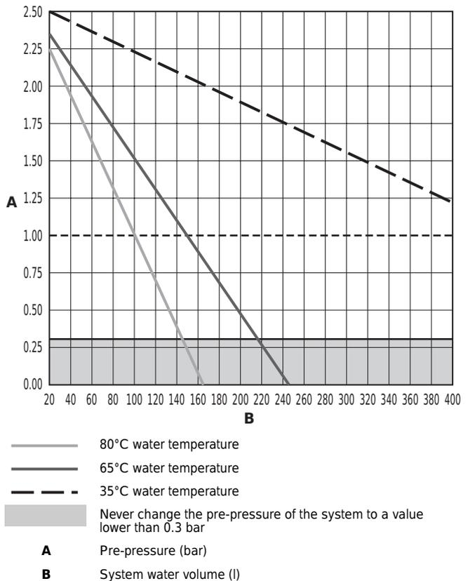
How to check if the pre-pressure of the system needs to be changed:
