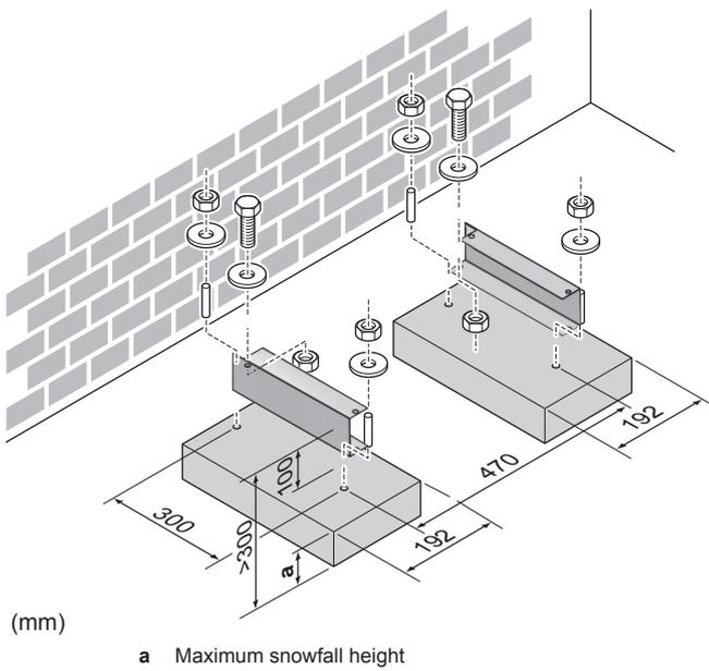
If the unit is installed on brackets to the wall, install the unit as follows:
