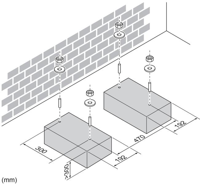
In any case, provide at least 300 mm of free space below the unit. Additionally, make sure the unit is positioned at least 100 mm above the maximum expected level of snow. In this case, it is recommended to construct a pedestal.
